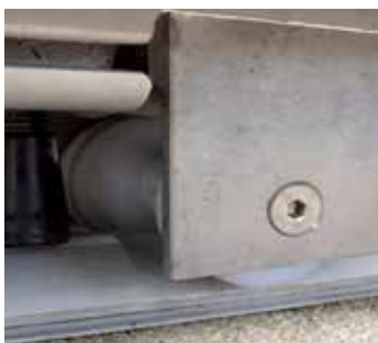
Brake with rubber pad and guide wheel
